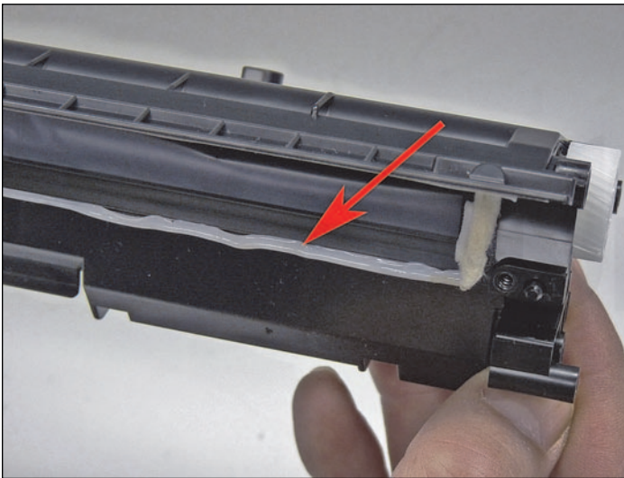
24. Clean out any remaining toner from the hopper. Note the doctor blade seal. It is a sticky substance that can be clean with alcohol if toner gets on it. If this seal becomes damaged, replace it with 100% silicon caulk.
