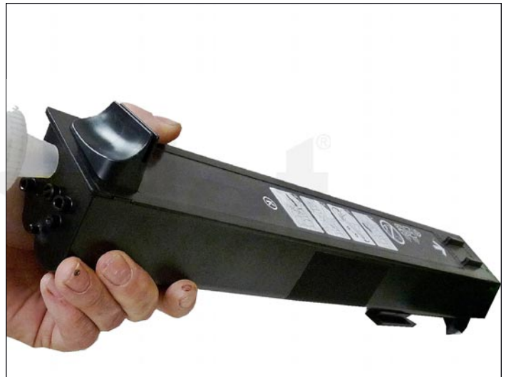
6. Clean all the remaining toner, and fill with new replacement toner for use in the M855 and M880 printers.
