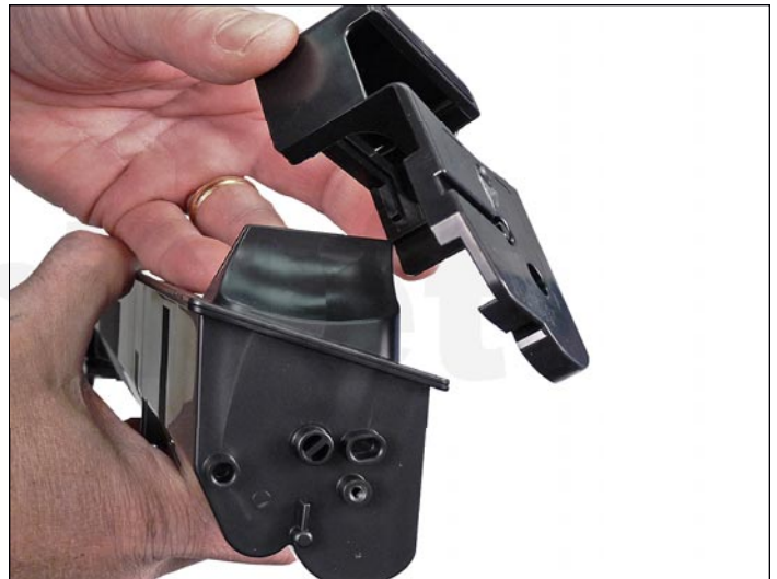
4. Press in on the middle curved section and slide the cover up and off of the cartridge.
