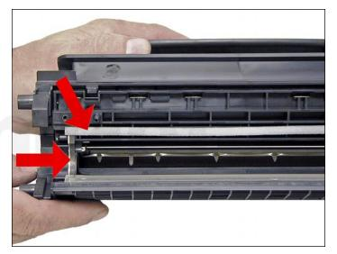
27. Note the magnetic seals on the MRS and the doctor blade sealing foam. Make sure both are clean.
