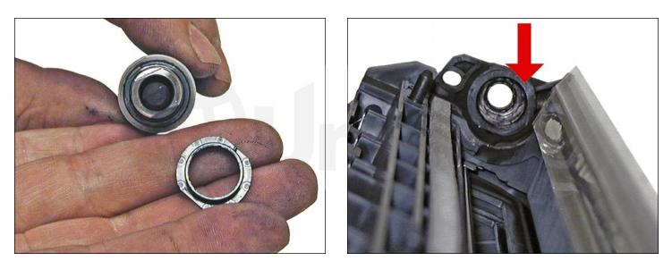
29. There are magnetic roller bushings on each side of the roller.
