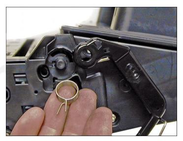
3. On the opposite side of the cartridge, carefully pry off the drum cover plastic arm. The spring will probably pop off, so take care not to lose it. We will go over the installation at the end of this article. Remove the drum cover assembly.
