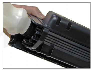
38. Fill with appropriate amount of toner for use in the M630 series. Install the fill plug.
