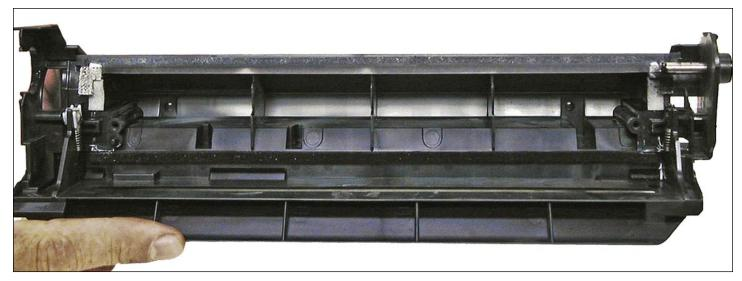
14. Due to the high speed and page counts of these cartridges, we recommend that the wiper blades be replaced.
