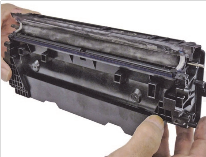
28. Install the feed roller, pointed-end to the open side.
