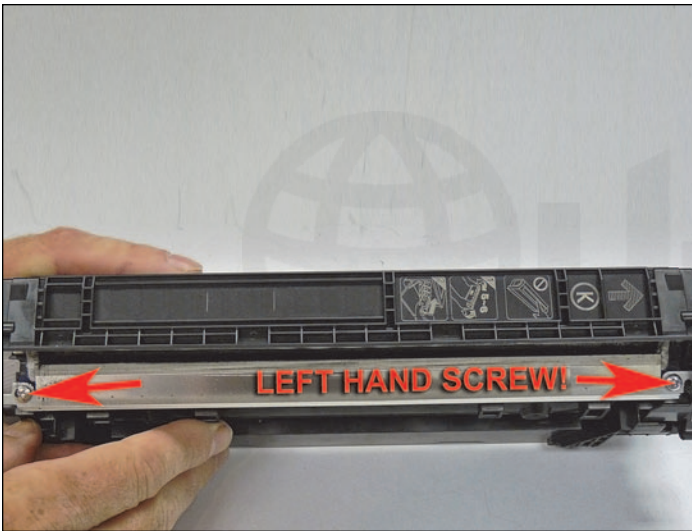
21. Remove the two screws from the doctor blade.
