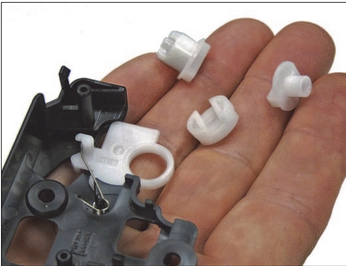
19. Remove the three developer roller drive gears.
