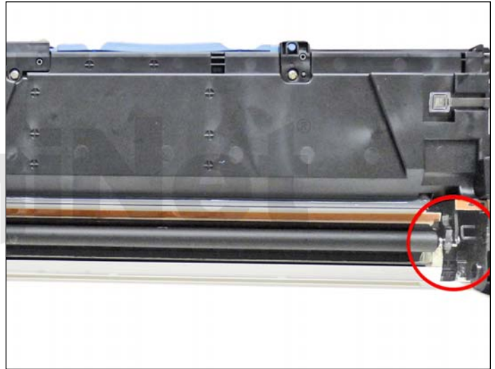
22. Clean the PCR and install the PCR assembly. Be careful not to damage the film. Replace the conductive grease on the black holder side of the PCR.
