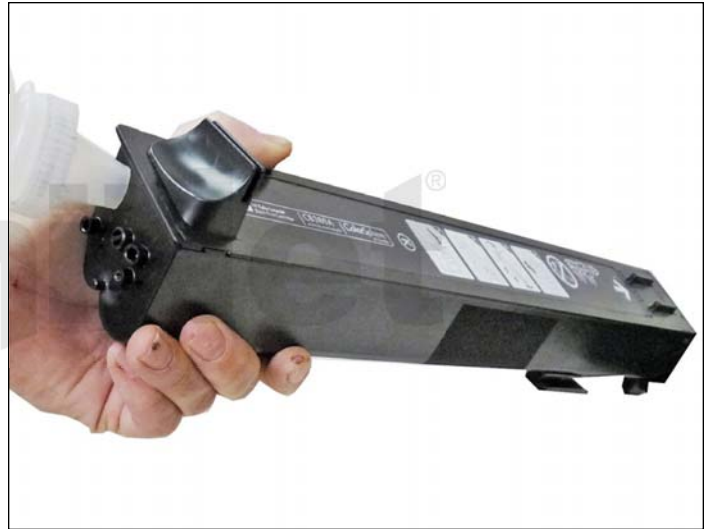
6. Clean all the remaining toner and fill with dedicated toner for HP CP6015.
