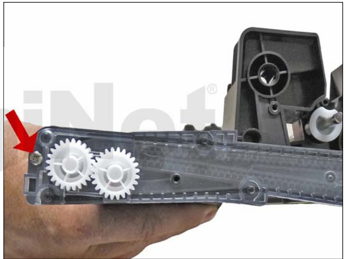
7. Remove the single screw and belt/gear train.
