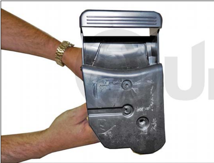
15. Slide the fill side end cap in place. Install the screw and replace the label (the label as you can see is easily torn).
