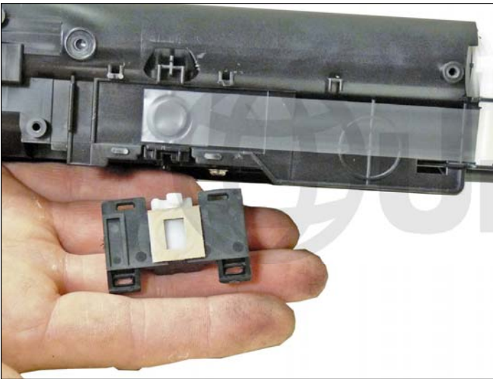
11. Remove the seal cover by carefully prying it off.
