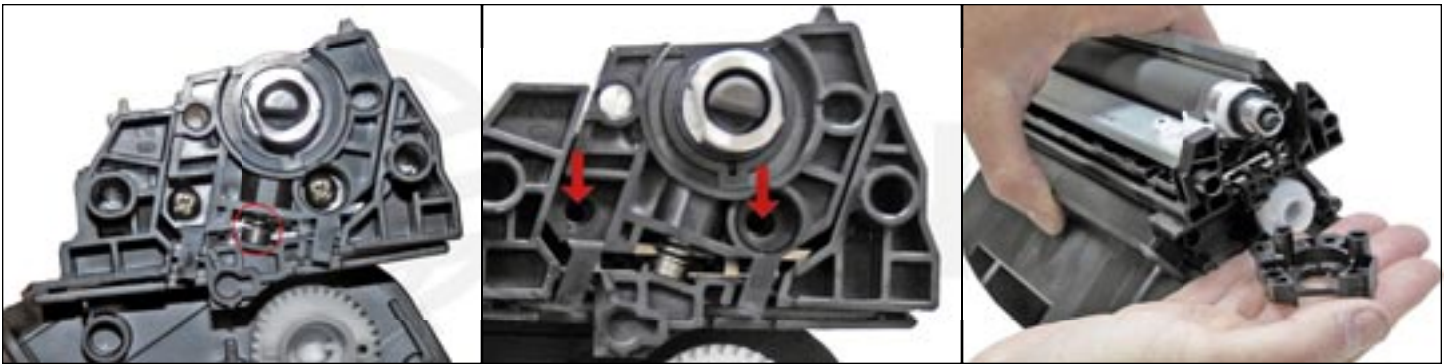
19. Note the location of the spring that sits between the magnetic roller sleeve holder and the hopper.
