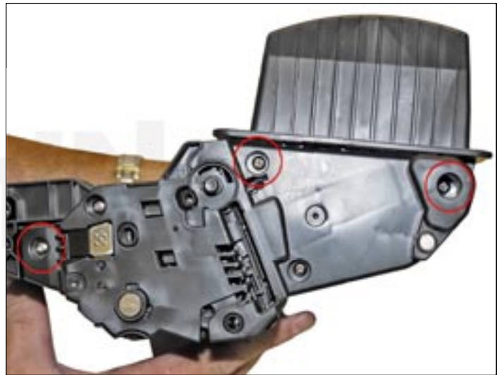
35. Install the remaining three screws on the left-side end cap.
