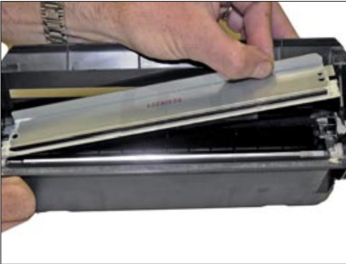
12. Note that there is not any type of sticky sealant on the wiper blade. There is just normal foam and felt seals under the blade. Remove the wiper blade from the cartridge, and clean out the waste toner. Be careful not to damage the spring coming out from the black PCR holder. Clean the PCR with your standard PCR cleaner.
