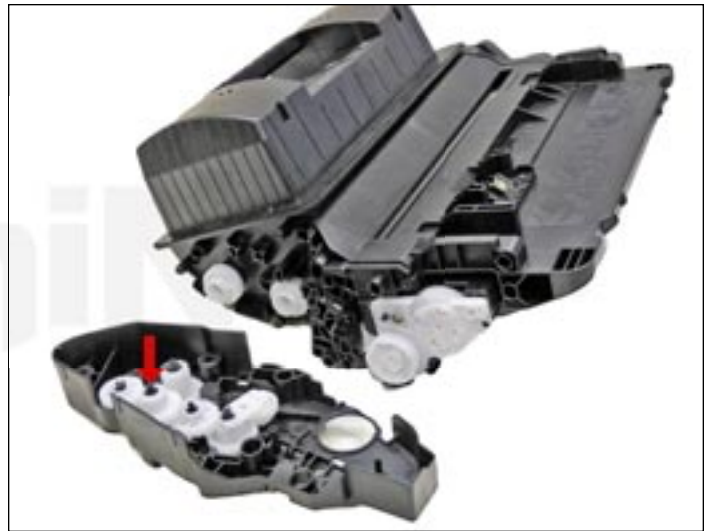
6. Remove the right-side end cap from the cartridge.
