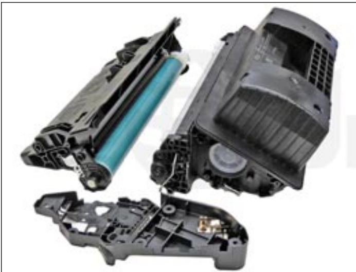
7. Remove the left-side end cap. Both halves will come apart easily. Be careful not to damage the drum or magnetic roller sleeve.
