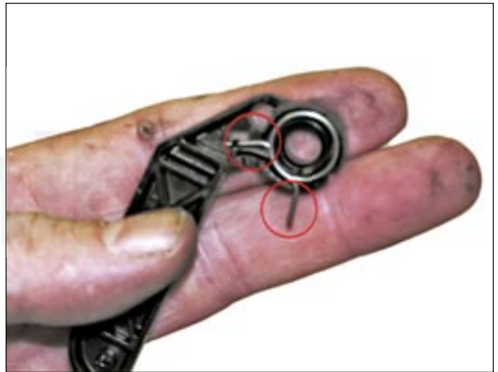
37. Install the spring into the drum cover arm as shown. Pull the upper tail of the spring until it fits into the notch in the arm hub.
