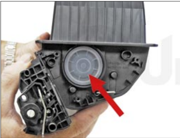
22. Remove the fill plug from the hopper.
