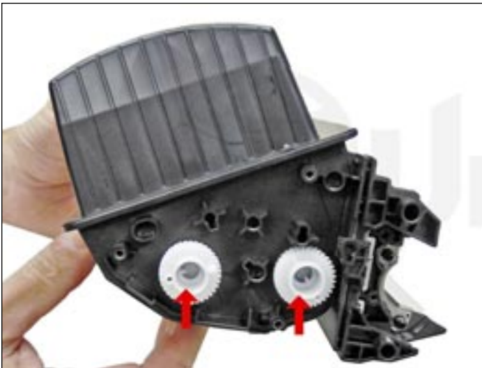
24. There are two separate mixing blades in the toner hopper. The largest is on the bottom, with the smallest on the top. Each is driven by its own separate drive gear. The upper magnetic roller section of the toner hopper “floats” on a series of foam seals. The upper half can be removed from the hopper, but some of the seals will be destroyed. This may become necessary in order to seal the cartridge. We will keep you informed on the availability of a seal system and how to install it as our testing continues. The foam isolates the magnetic roller from the vibrations of the mixing augers, and allows smoother prints.
