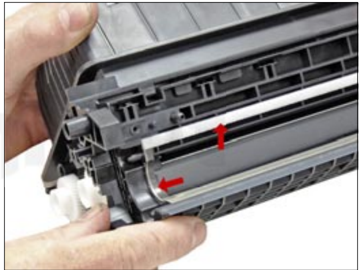
23. Note the magnetic seals on both the magnetic roller sleeve and doctor blade sealing foam. Make sure both are clean.
