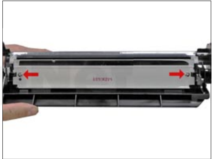
11. Remove the two screws from the wiper blade. Due to the high speed and page counts of these cartridges, we recommend that the wiper blades be replaced.
